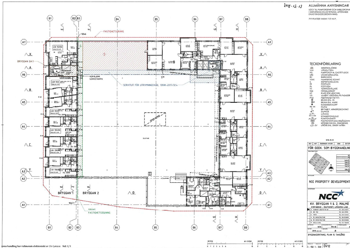
Figure 8. Example of computer aided design (CAD) construction plans in Multihuset as part of the actual property formation dossier, green lines representing property boundaries (Source: NCC Company).
